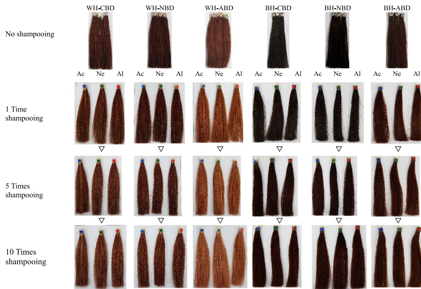
Fig. 3 White hair (WH) and bleached hair (BH) dyed with Cationic (CBD), Nonionic (NBD), and Anionic (ABD) basic hair dye before and after up to 10 times of shampooing. Ac acidic shampoo, Ne neutral shampoo, Al alkaline shampoo
