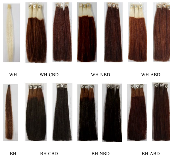
Fig. 1 White hair (WH) and bleached hair (BH) after dyeing with Cationic (CBD), Nonionic (NBD), and Anionic (ABD) basic hair dyes
