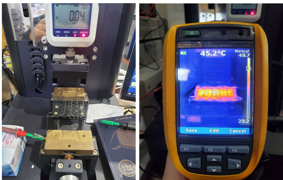
Fig. 4 Measuring driving force of real shape memory textile actuator with Universal Testing Machine
