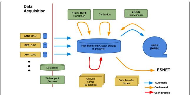
Fig. 2 Logic diagram of the LCLS data management system. The blue arrows indicate data movement that is automatically handled by the DM system; the red arrows indicate traffic that is handled by the users; the red arrows show traffic that is handled by the DM system upon users' request
