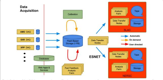
Fig. 7 Evolution of the LCLS data systems architecture. The data management system will transparently integrate external supercomputers from facilities like NERSC
