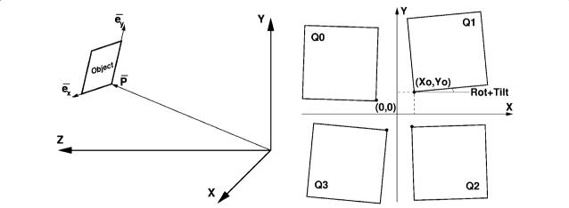
**Fig. 5** Hierarchical geometry description used by psana. *Left* one level in the hierarchical geometry description used by psana showing a child object in the parent coordinate frame. *Right* several panels of a multi-panel detector showing rotations and offsets. Although not shown in the diagram, the hierarchical geometry description allows these to be out-of-plane
