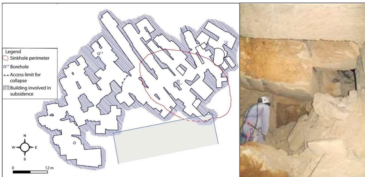
Fig. 15 On the left: topographic survey of the underground quarry before failure, with indication of the sinkhole perimeter (Bonamini et al. 2013). On the right: movements of large volumes of rock along sub-vertical fractures surveyed in 2000 (Vattano et al. 2013)
