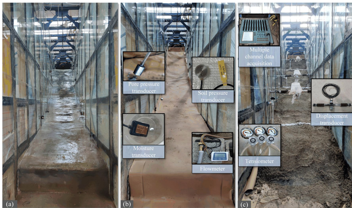
Fig. 8 Model building process a Sliding bed fabrication, b sliding surface production, c sliding body fabrication
