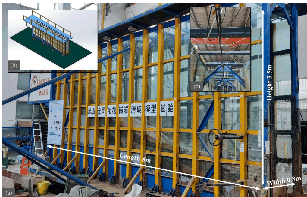
Fig. 6 a , b Model overview, c rainfall device
