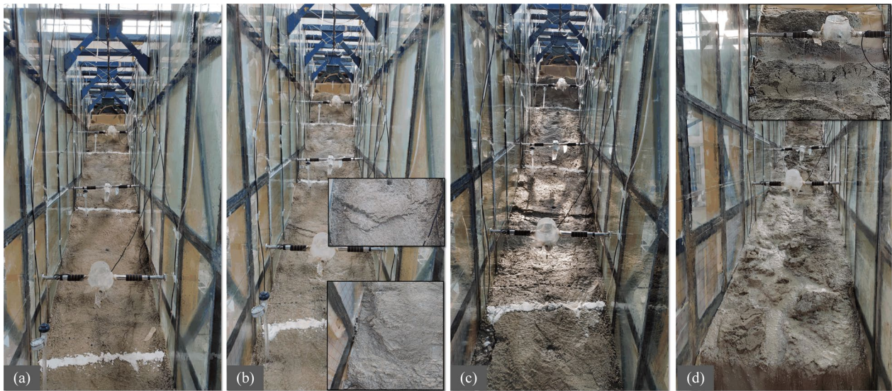
Fig. 15 Landslide deformation process under condition N1 a 0.1 h, b 0.3 h, c 0.5 h, d 0.9 h
