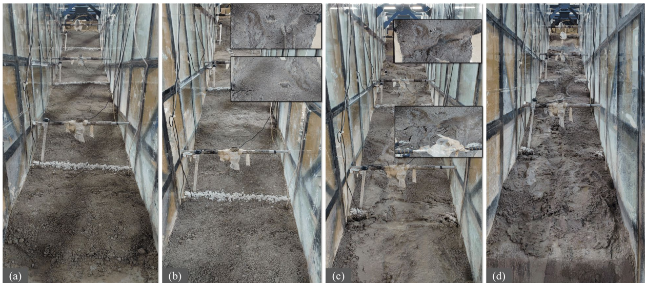
Fig. 16 Landslide deformation process under condition N2 a 0.1 h, b 0.3 h, c 0.9 h, d 1.1 h
