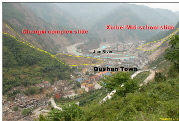
Figure 4 The Chengxi complex landslide (left) and the Xinbei Mid-school rockslide (right) in Qushan Town, Beichuan County. The Chengxi landslide killed 1,600 people and the Xinbei Mid-school rockslide killed 500 people. The dotted lines show the travel path and the extent of each landslide.
