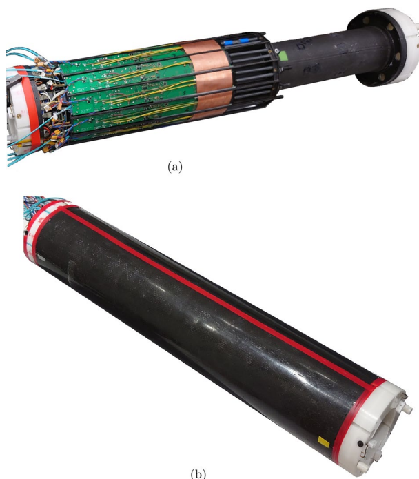
Fig. 2 Photographs of the open and closed SAFIR-I detector. Photography by P. Bebié
