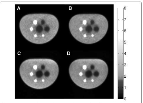
**Fig. 3** 2D cross-sections of reconstructed image quality phantom at the axial center of the spheres with a 192 × 192 image matrix. The ratios of the activity concentrations within hot rods, background, and cold rods were 8:1:0. **a** 3D-OSEM. **b** 3D-OSEM with PSF function. **c** 3D-OSEM with TOF information. **d** 3D-OSEM with both TOF information and PSF function
