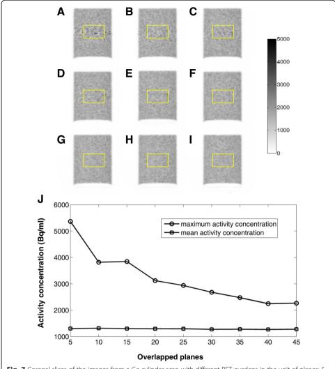
**Fig. 7** Coronal slices of the images from a Ge cylinder scan with different PET overlaps in the unit of planes: 5 (a), 10 (b), 15 (c), 20 (d), 25 (e), 30 (f), 35 (g), 40 (h), and 45 (i). The emission data were acquired for a total of two bed positions. **j** Maximum and mean value of activity concentration as a function of overlapped planes
