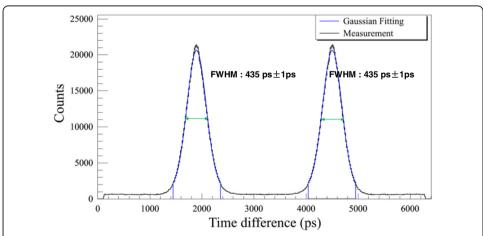
**Fig. 1** The true timing spectrum acquired using a rotating line source that orbits around the CFOV at a radius of 20 cm. Gaussian fitting was applied to the two peaks, and the average FWHM was reported as the timing resolution of the system
