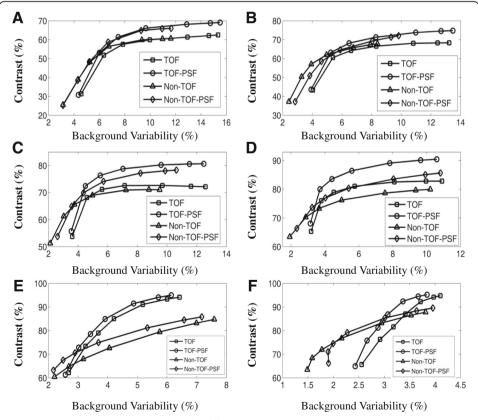
**Fig. 10** Contrast vs background variability for different reconstruction algorithms (TOF, TOF+PSF, non-TOF, and non-TOF+PSF) and a number of iterations (points of each graph correspond to 1, 2, 3, 5, 10, 15, and 18 iterations). These plots are used to estimate the performance balance for hot rods with an inner diameter of 10 mm (**a**), 13 mm (**b**), 17 mm (**c**), and 22 mm (**d**) and cold rods with an inner diameter of 28 mm (**e**) and 37 mm (**f**)
