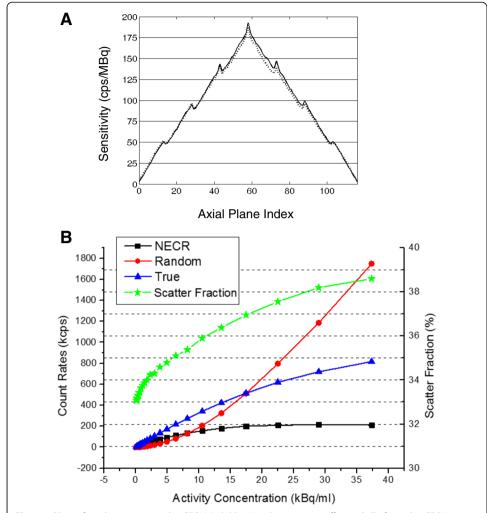
**Fig. 2 a** Plots of axial sensitivity at the CFOV (solid line) and at a 10-cm offset radially from the CFOV (dotted line). **b** Plot of NECR (square), randoms (circle), true (triangle), and scatter fraction (star) as a function of activity concentration
