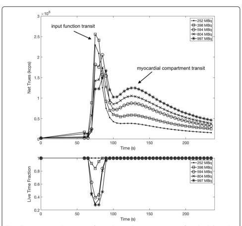
**Fig. 4** Top—Net trues and prompt rates from each injected activity experiment performed with the cardiac perfusion phantom. Of note is that above a net trues rate of approximately  $2.6 \times 10^6$  (corresponding to  $A_{\rm INJ} = 398$  MBq), the trues rate at peak input function actually begins to decrease due to the decrease in live-time fraction
