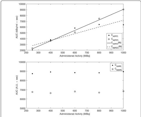
**Fig. 6** Area under the curves for (top)  $C_{A(\text{PET})}$ ,  $C_{M(\text{PET})}$ , (bottom)  $C_{A(\text{MR})}$  and  $C_{M(\text{MR})}$ . AUC increase linearly for  $C_{M(\text{PET})}$  up to  $A_{\text{INJ}} = 997$  MBq ( $R^2 = 0.99$ ), whereas the effect of count losses is observed for  $C_{A(\text{PET})}$  ( $R^2 = 0.72$ ). Repeatability measurements are shown by  $C_{A(\text{MR})}$  and  $C_{M(\text{MR})}$
