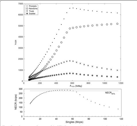
**Fig. 1** Top—Count-rate performance of the PET-MR system with activity present in the myocardial chamber of an anthropomorphic torso phantom. Of note is a discontinuity in the response at a maximum prompt rate of 6596 kcps (corresponding to a singles rate of 64.9 Mcps), above which events become affected by counting losses. Bottom—Noise equivalent count rate (NECR), with a peak rate of 286 kcps at a singles rate of 47.1 Mcps, and NECR<sub>95%</sub> of 34.1 Mcps
