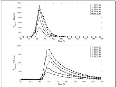
**Fig. 5** Time-activity curves resulting from image analysis with increasing activity administrations to the phantom. Top:  $C_{A(\text{PET})}$ , and bottom:  $C_{M(\text{PET})}$ , showing input and washout of the radiotracer.  $C_{A(\text{PET})}$  for 804 and 997 MBq injected activities do not increase at the same rate as the myocardial TAC suggesting the reconstructed images are affected by count losses
