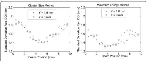
**Fig. 14** Standard deviation of the reconstructed depth of interaction using the cluster size method (*left*) and the maximum collected energy method (*right*)
