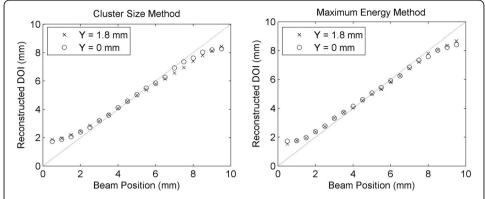
**Fig. 13** Reconstructed depth of interaction as a function of the collimated beam position (*Z* direction) using the cluster size method (*left*) and the maximum collected energy method (*right*). The line in the plots represents the bisector of the plane, corresponding to an ideal reconstruction of the beam position
