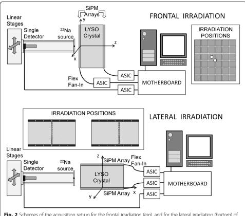
**Fig. 2** Schemes of the acquisition set-up for the frontal irradiation (*top*), and for the lateral irradiation (*bottom*) of the detector (not to scale). The reference axes and the irradiation position are reported in the two configurations
