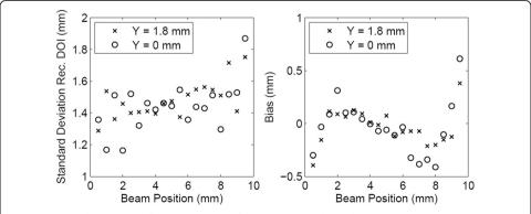
**Fig. 16** Standard deviation (*left*) and bias (*right*) of the reconstructed DOI distributions using the combination of the two asymmetry parameters and the calibration obtained with the lateral scan of the detector
