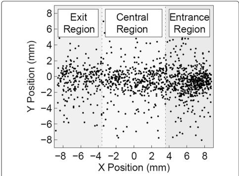
**Fig. 5** Example of the distribution of the events in the *X-Y* directions for a lateral irradiation at the center of the module. The three regions used for the analysis of the DOI determination capabilities are represented in figure
