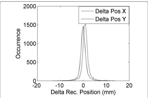
**Fig. 4** Difference in the reconstructed *X* positions (*continuous line*) and *Y* positions (*dotted line*) on the two faces of the crystal. Positions were reconstructed separately on the two sides using the center of gravity method on the SiPMs of the cluster
