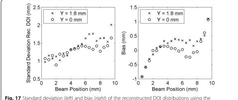
**Fig. 17** Standard deviation (*left*) and bias (*right*) of the reconstructed DOI distributions using the combination of the two asymmetry parameters and the calibration obtained with the <sup>176</sup>Lu background
