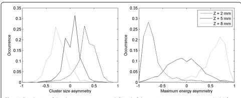
**Fig. 12** Distribution of the cluster size asymmetry (*left*) and of the maximum energy asymmetry (*right*) for the points [2 mm, 5 mm, 8 mm], in the scan at the center of the lateral surface
