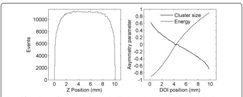
**Fig. 6** (*left*) Distribution of the centroid of the simulated background events in the Z direction. (*right*) Cluster size asymmetry (*solid line*) and maximum energy asymmetry (*dashed line*) calibration function obtained correlating the simulation with the acquisition of the  $^{176}$ Lu background
