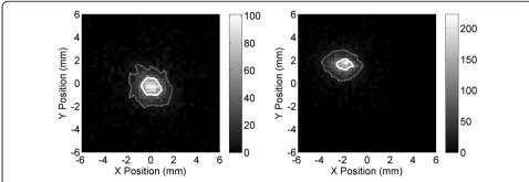
**Fig. 8** Spatial distributions obtained with the collimated beam at the center of the detector (*left*) and at 1.8 mm from the center in both directions (*right*), corresponding to the center of one of the SiPM of each matrix. Continuous lines represent the contour corresponding to the FWHM of the distribution while dotted lines correspond to the FWTM of the distribution
