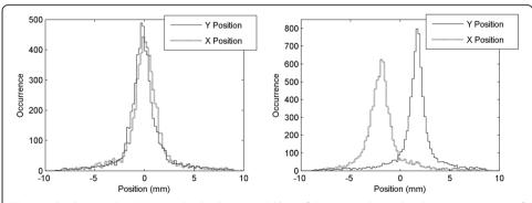
**Fig. 9** *X* distribution (*dotted lines*) and *Y* distribution (*solid line*) of the events obtained in the two acquisitions of Fig. 8, with the coincidence beam at the center of the crystal (*left*) and at 1.8 mm from the center in both directions (*right*)
