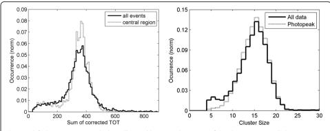
**Fig. 10** (*left*) Energy spectra with the collimated beam at the center of the detector using all the events (*continuous line*) and only the events inside the FWHM of the distribution (*dotted line*). (*right*) Total number of SiPMs in the clusters in the two sides of the detector for the whole data-set (*solid line*) and for the photopeak events selected in the energy window (*dotted line*)
