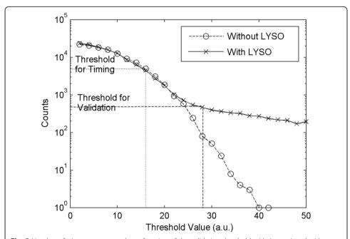
**Fig. 3** Number of triggers per second as a function of the validation threshold with (*crosses*) and without (*open circles*) the scintillator coupled to the SiPM. The threshold values to trigger the time stamp and to validate the events are shown (*dashed lines*)
