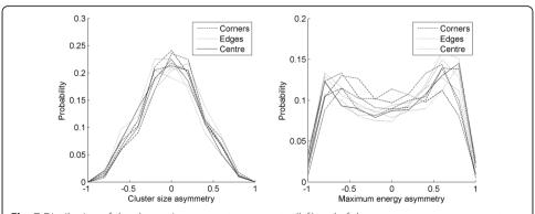
**Fig. 7** Distribution of the cluster size asymmetry parameter (*left*) and of the energy asymmetry parameter (*right*) for different regions of the detectors corresponding to the four edges, the four corners and the central region, obtained with the natural <sup>176</sup>Lu background
