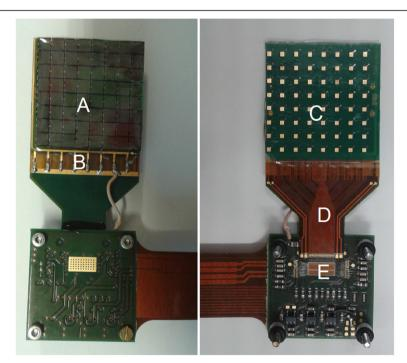
**Fig. 1** Picture of the SiPM matrix coupled to the PCB containing the ASIC. (*left*) The SiPM array (**a**) receives the bias from the pads on the top side through a bonding chain connected to the bias in the PCB (**b**). (*right*) On the back side, each channel is connected to a pad (**c**) used to probe the signal during the functionality test, and is collected in a fan-out (**d**). A flex cable connects the array to the ASIC (**e**)
