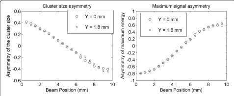
**Fig. 11** Cluster size asymmetry (*left*) and energy asymmetry (*right*) obtained in the lateral *Z* scans at the center of the lateral surfaces (*circles*) and at 1.8 mm from the center (*crosses*)
