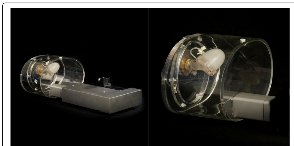
Fig. 2 The AGATE dynamic gated phantom. The AGATE dynamic gated phantom with fillable cardiac set, successively filled with a solution of ^{123}\text{I} alone, ^{99\text{m}}\text{Tc} alone, and a mixture of ^{123}\text{I} and ^{99\text{m}}\text{Tc}
