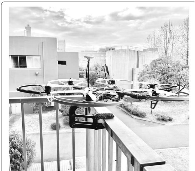
Fig. 1 Multicopter with simple underactuated device can perch on veranda easily for delivery, security monitoring, etc.
