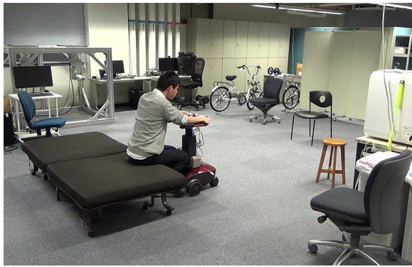
Fig. 11 Experimental setup. Participants sit and stand from all chairs and bed using the robot
