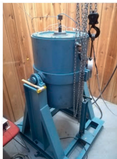
Fig. 4 Schematic diagram of an internally heated pressure vessel with rapid quench device (left) and a rapid quench IHPV at Bayerisches Geoinstitut (right, modified from Yoshioka 2018)
