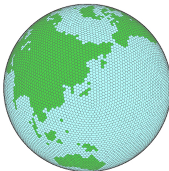
Fig. 21 Model grid of the “glevel-5” NICAM. The mean grid interval is ca. 223 km (Satoh et al. 2014)
