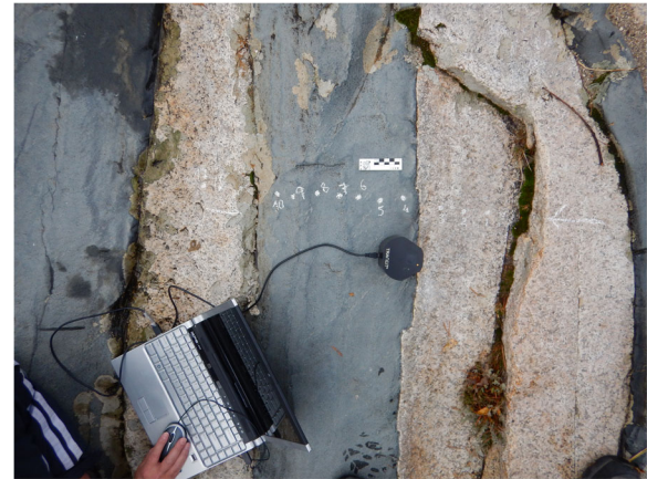
Fig. 4 Innovep TraceIT optical rugosimeter. The acquisition unit (centre) contains the three collimated light beams and cameras that allow a photogrammetric reconstruction of a 5 \times 5 mm area. North is on the right of the image
