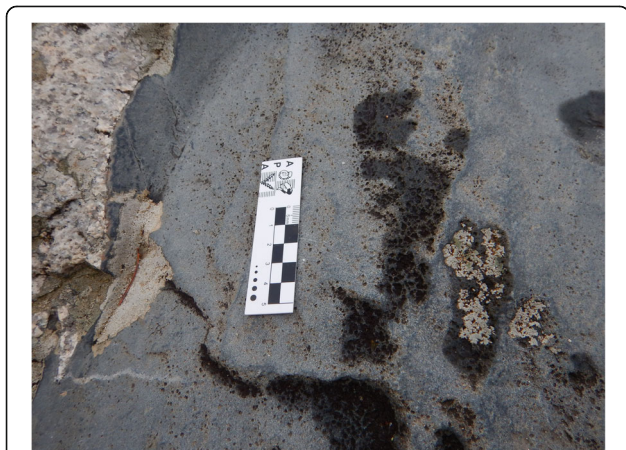
Fig. 3 Millimetre-scale pits and grooves in a microdiorite dyke. Dark-coloured area corresponds to moisture accumulated in and around pits. This is likely to cause weathering through wetting-drying cycles
