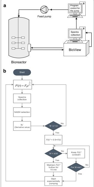
**Fig. 1 a** Schematic overview of the bioprocess setup of the fedbatch cultivations with the feedback control. **b** Overview flowchart of the feed rate control
