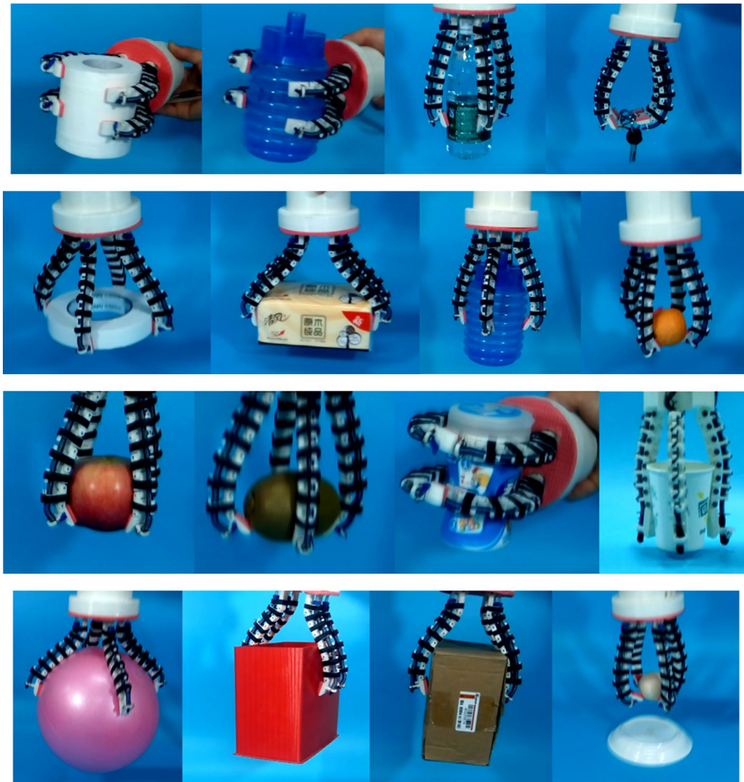
Fig. 12 Experiments of OS Hand with for tentacles
