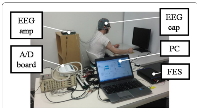
Fig. 3 Overview of the system. An EEG cap is set on the patient's head. EEG data are measured by the EEG cap, amplified by the EEG amp and output via the A/D board to a PC. The PC is used to analyze the EEG data and actuate the FES
