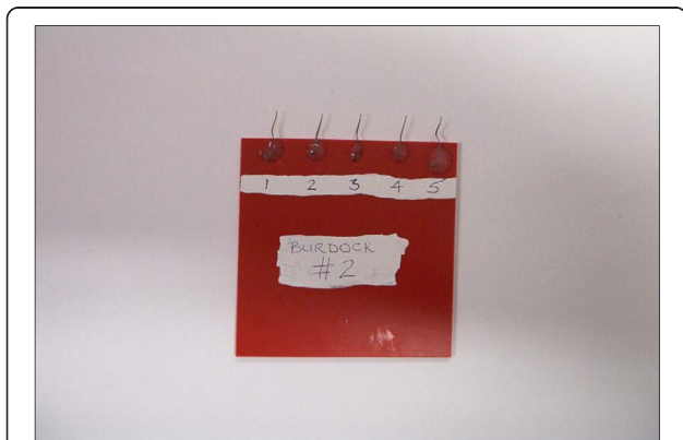
Fig. 2 Hooks mounted in preparation for testing in the Instron machine by gluing each separate bract to a plastic mounting
