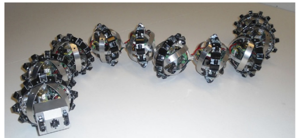
Figure 2 An illustration of the experimental setup. Snake robot Wheeko was used for the experiments.
