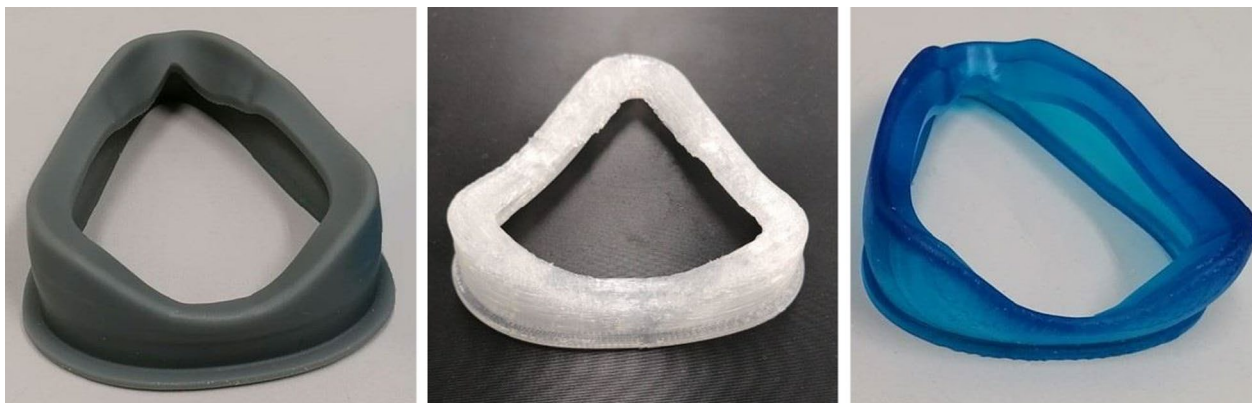
Fig. 2 An overview of the personalized cushion materials. From left to right: silicone urethane (SU) printed on a DLS printer, silicone (Si) printed on an FDM printer, and soft photopolymer resin (SPR) printed on a DLP printer
