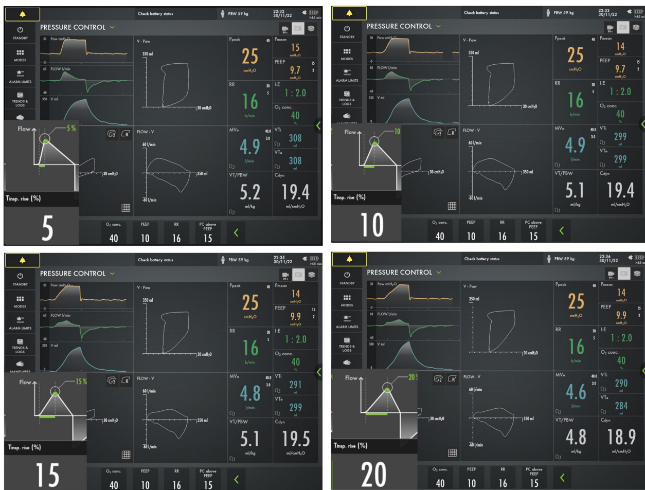
Fig. 4 Dynamic pressure–volume loop (P–V), pressure–time, flow–time and volume–time graphics of I:E 1:2 and T_{slope} 5%, 10%, 15% and 20% in PCV mode (obtained with screen shots of the Servo-U mechanical ventilator)
