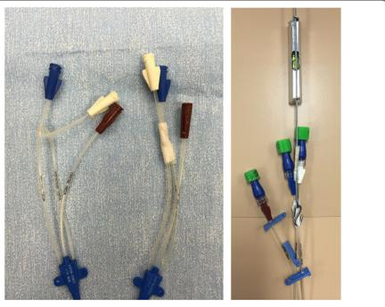
Fig. 3 Lumens tied in a knot and taped; IMASS hook placement on lumens for pull test
