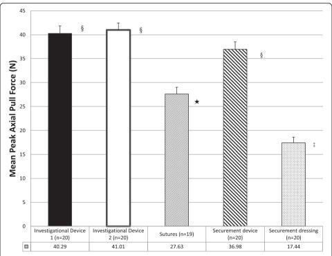
Fig. 5 Mean peak axial pull force for each type of securement device (least squares, mean ± standard error). Samples labeled with the same symbols are not significantly different from each other. Least squares means differ slightly from the unadjusted means displayed in Table 2 due to the overall imbalance of securement devices placed on pigs
