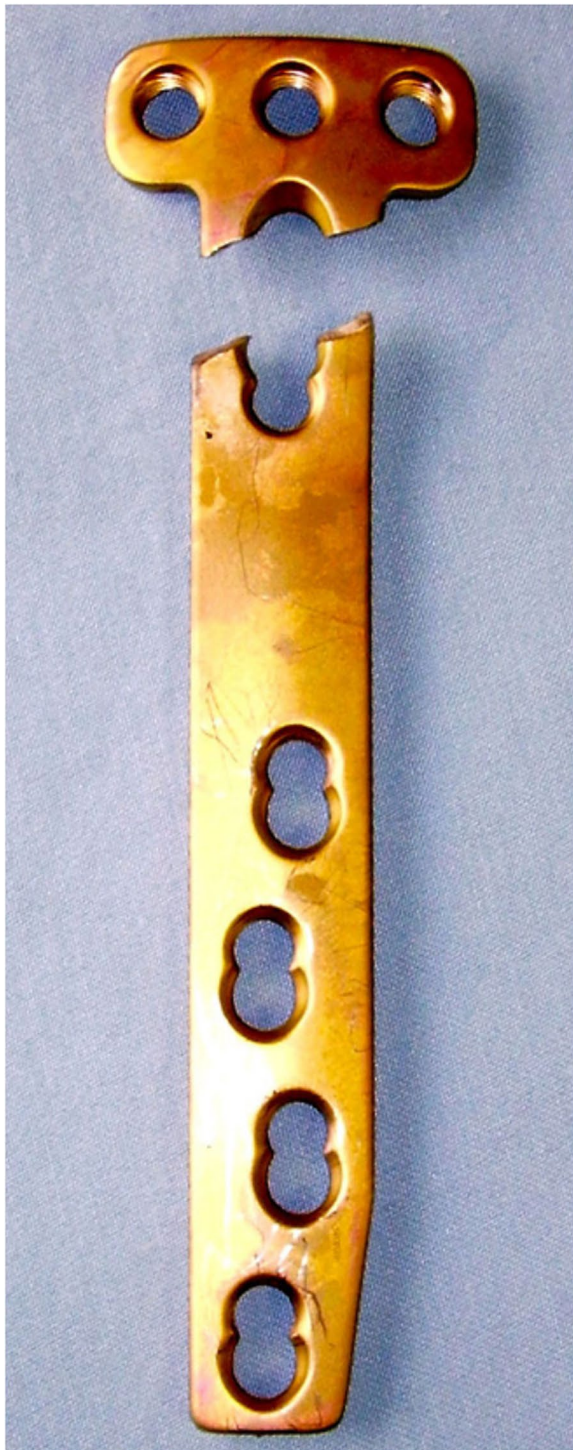
Fig. 5 Fracture of a plate fixator (Tomo-Fix, Depuy-Synthes) due to lack of occupation of the "D-hole". This has led to too high a load concentration on the plate in this area and ultimately produced the plate fracture
