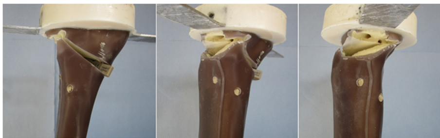
Fig. 9 Fracture of the contralateral cortex (specimen with the iBalance implant). The opposite cortex appeared to be the weak point of the bone-implant constructs
