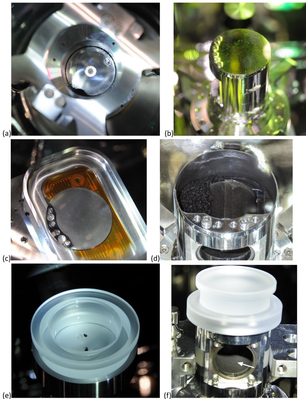
Fig. 14 a An image of the bottom of the HY2 sampler container. A certain amount of sample grains are visible. b A photograph of the surface of Chamber A of the sample catcher. Fine powdery grains are observed clearly by the illumination with a green LED light, which is useful in recognizing fine dust on the surface of materials. c An image of the cover of chamber A of the sample catcher attached on the surface of the electrostatic chuck in CC3-2. The inner surface of the chamber A of the catcher is covered with very fine powdery samples as the reflection on the surface was vague. d An image of sample grains in the chamber A of the sample catcher. This is referred from Fig. 1 of Clark (2022). e An image of a few sample grains of mm-size, which are preserved in the quartz glass container under the vacuum condition in CC3-2 to date. f An image of the powdery samples (pointed by a white arrow) inside the rotation cylinder of the sample catcher situated at the stage 4 in CC3-3. This was shot when the handling jig was about to be attached
