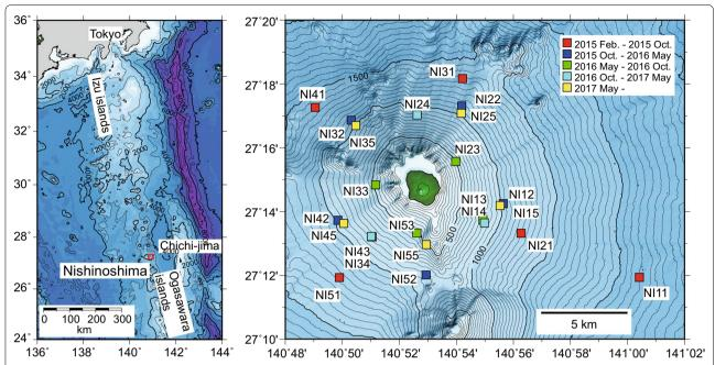
**Fig. 1** Index map of Nishinoshima (left) and positions of LT-OBSs around Nishinoshima (right). Left: Nishinoshima is part of the Izu-Ogasawara volcanic arc system and is positioned approximately 1000 km south of Tokyo. Right: squares indicate positions of LT-OBSs, deployed from February 2015 to May 2017. Observations were divided into four terms, which are classified in terms of colors. Bathymetry was obtained by JCG (Morishita et al. 2017). Contour intervals for bathymetry is 20 m
