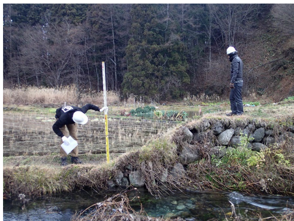
Fig. 2 An example of coseismic surface offset due to reverse faulting. Photograph taken at a site called Joyama located in the central part of the focal area. View from the south
