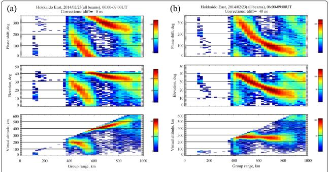
**Fig. 7** Two-dimensional histograms of the phase (*top*), elevation (*middle*) and virtual height (*bottom*) vs range calculated for the 06–09UT interval from Fig. 6 but using all radar beams: **a** the original (uncorrected) data; **b** data corrected with *tdiff* = 40 ns
