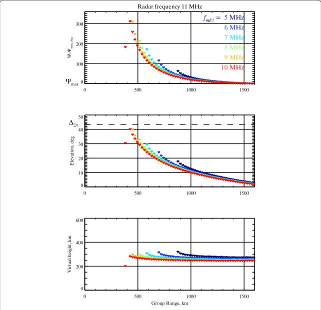
**Fig. 4** Simulated phase shift (*top*), elevation (*middle*) and virtual height (*bottom*) variations vs group range for the reflection points of ground scatter in Fig. 3. The data were processed in the way that resembles operation of SuperDARN radars with a 45-km group range resolution (see text for more details)
