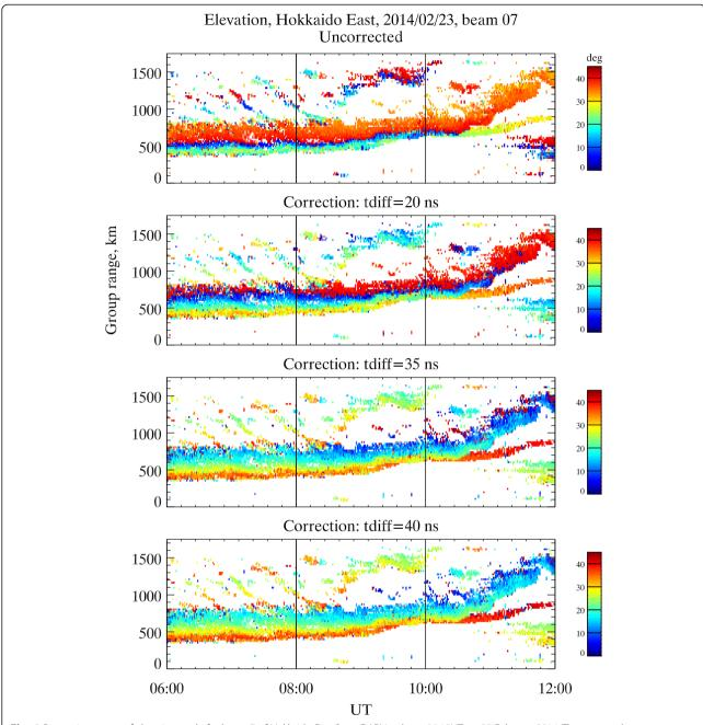
Fig. 6 Range-time maps of elevation angle for beam 7 of Hokkaido East SuperDARN radar at 06-12UT on 23 February 2014. The top panel represents uncorrected data, while the remaining three panels show elevation values with a gradually increasing (top to bottom) correction time offset, tdiff
