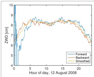
**Fig. 1** ZWD estimated at Ny-Ålesund, Spitsbergen, Norway, with the Kalman filter on 12 August 2008. Shown are the results from the forward running Kalman filter, the backward running Kalman filter, and the smoothed results
