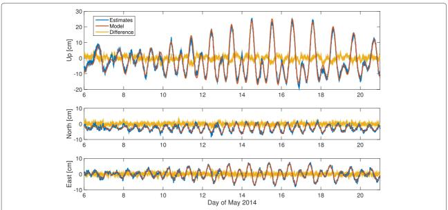
**Fig. 6** Estimated position variations of the YEBES40M station during CONT14, together with the predicted variations from the solid Earth tide model in the IERS 2010 Conventions. No solid Earth tides were applied a priori
