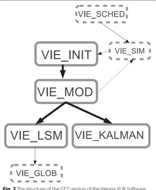
$\label{eq:Fig.2} \textbf{Fig. 2} \ \mbox{The structure of the GFZ version of the Vienna VLBI Software,} \\ \mbox{VieVS@GFZ}$
