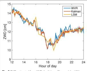
Fig. 5 ZWD estimated from WVR, the Kalman filter, and the LSM solution at Onsala on 14 August 2008 between 12:00 and 24:00 UTC
