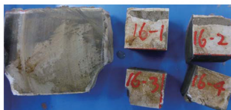
Figure 3 Photographs showing the samples used for archeointensity (paleointensity) and rock magnetic experiments. (a) An original cube sample (approximately 3.7 cm on a side) is vertically cut into two pieces. One is reserved as an archive while the other is further cut into several mini specimens for archeointensity (paleointensity) and rock magnetic experiments. Example photographs are shown for sample 1 from the floor surface. (b) An example photograph for sample 5 from the floor surface. (c) An example photograph for sample 16 from the -20-cm level.
