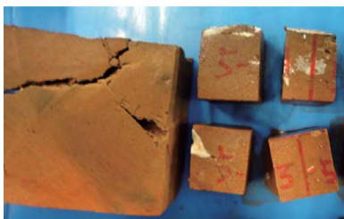
Figure 3 Photographs showing the samples used for archeointensity (paleointensity) and rock magnetic experiments. (a) An original cube sample (approximately 3.7 cm on a side) is vertically cut into two pieces. One is reserved as an archive while the other is further cut into several mini specimens for archeointensity (paleointensity) and rock magnetic experiments. Example photographs are shown for sample 1 from the floor surface. (b) An example photograph for sample 5 from the floor surface. (c) An example photograph for sample 16 from the -20-cm level.
