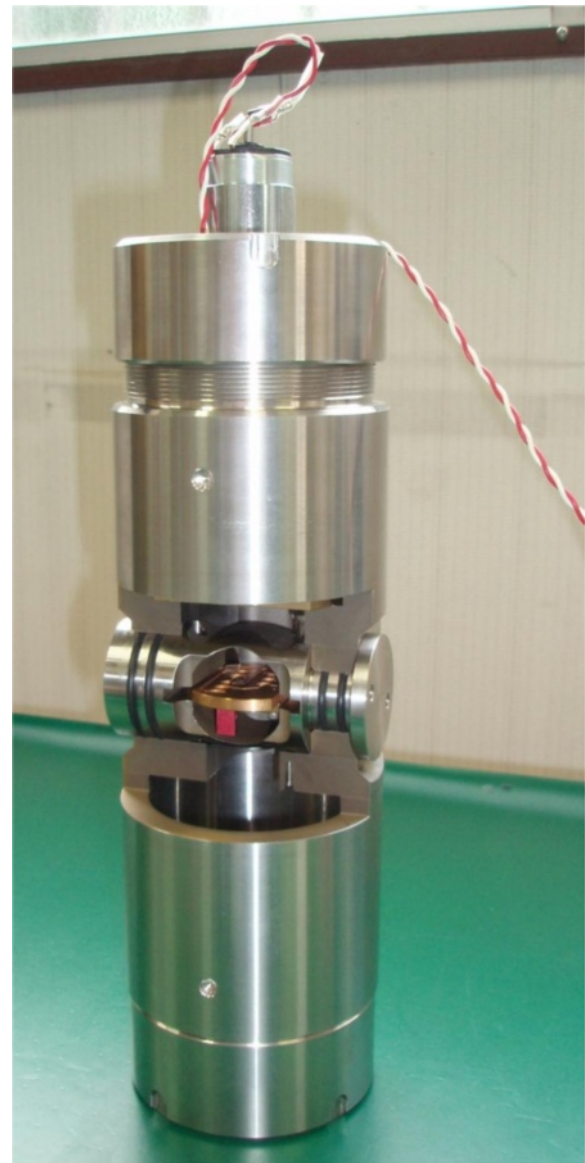
Figure 6 One horizontal component vessel where the stress sensing unit is installed. Half of the vessel is removed to show the installation of the sensing unit.
