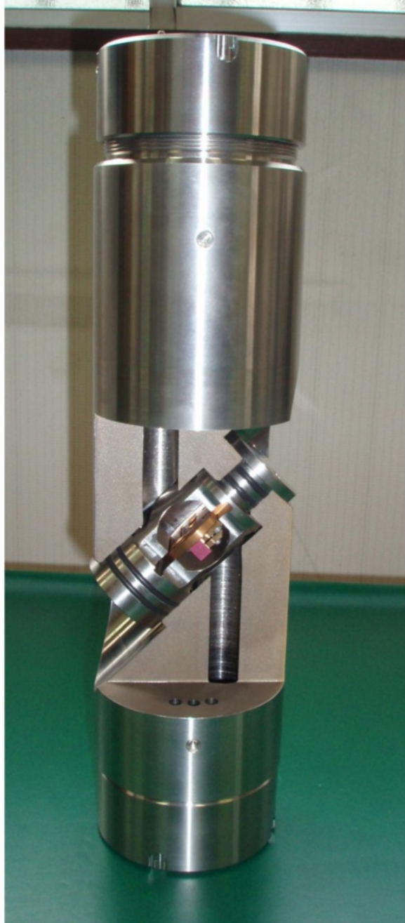
Figure 7 One inclined component vessel where the stress sensing unit is installed. Half of the vessel is removed to show the installation of the sensing unit.
