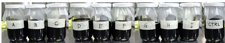
Fig. 1 Prepared ink formulation samples based on the mixture design for the three additives (wax, surfactant, defoamer)
