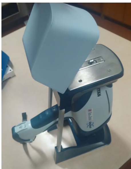
Fig. 1 The Bruker S1 Titan 600 ED-XRF spectrometer positioned vertically over the laboratory bench, with the help of an appropriate support. The shield box is rotated prior to analysis to avoid escape of X-rays
