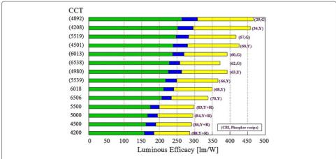
Figure 12 A comparison of the calculated limit of luminous efficacy of the pcW-LEDs in different phosphor recipes. The end of yellow bar is for LER, the end of blue bar is for limit of luminous efficacy of a pcW-LEDs, and the end of green is for the practical limit of the luminous efficacy.
