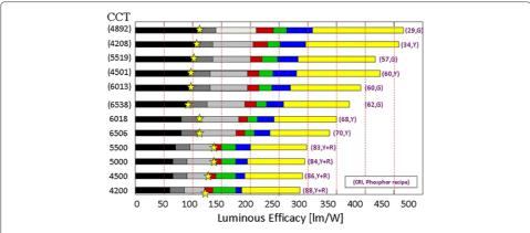
Figure 13 A comparison of the calculated limit of illumination luminous efficacy of the pcW-LEDs in different phosphor recipes. The right end of red bar is the luminous efficacy with 5% in electrical injection loss and 5% in thermal loss. The right ends of the light-grey, dark-grey and black bar are 90%, 60% and 45% in OUF, respectively, and respond to the applications in light bulb, automotive heal lamp and street light.
