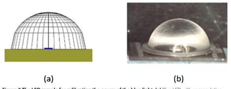
**Figure 2 The LED sample for calibrating the power of the blue light. (a)** Blue LED with encapsulation lens, and **(b)** the sample.
