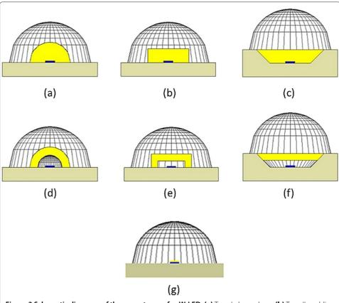
**Figure 3 Schematic diagrams of the seven types of pcW-LED. (a)** Type I, dome shape **(b)** Type II, molding **(c)** Type III, cup shape **(d)** Type IV, remote dome **(e)** Type V, remote molding **(f)** Type VI, remote cup **(g)** Type VII, conformal coating.
