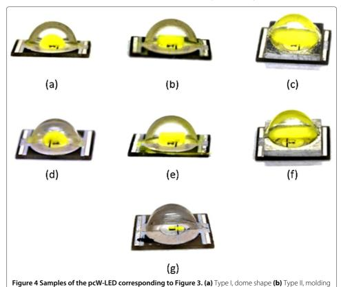
(c) Type III, cup shape (d) Type IV, remote dome (e) Type V, remote molding (f) Type VI, remote cup (g) Type
