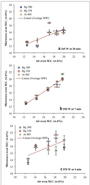
**Fig. 1** Apparent moisture contents (w.b.%) relationship of three different sizes of paddy varieties determine by air oven and domestic microwave oven-drying methods: **a** 265 W within 20 min drying, **b** 550 W within 7 min drying and **c** 870 W within 4 min of absorbed microwave drying
