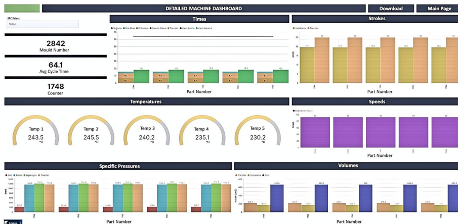
Fig. 10 Detailed machine dashboard shows near real-time process data such as pressure, time, volume, speed, and temperature. Plots on the dashboard are mostly grouped by part number. Users can compare different parts in terms of the process parameters by selecting part numbers using the drop-down menu on the left corner. This dashboard is refreshed automatically every 5 s
