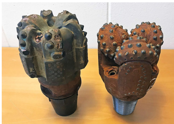
Fig. 5 Examples of the used drill bits in FFC-1. To the left, PDC (Z613) used between 2319 and 2338 m, and to the right TCI roller cone bit (637Y) used between 2413 and 2416 m. Photo J-E Rosberg
