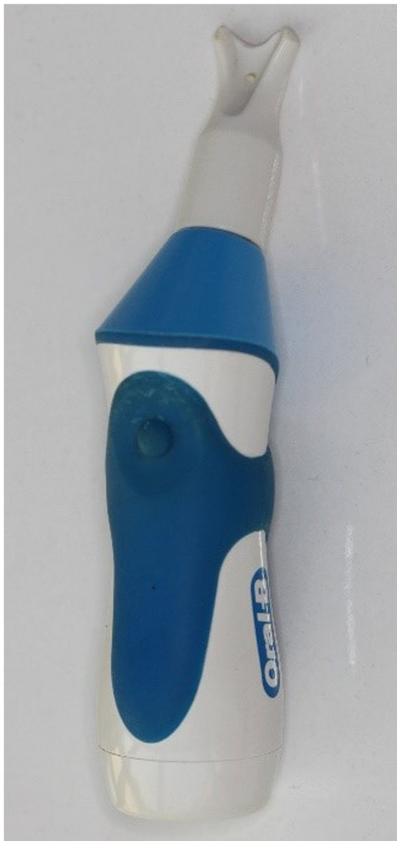
Fig. 2 Oral-B HummingBird device with a modified tip
