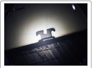
Fig. 2 Measurements of the brackets' slot with a profile projector
