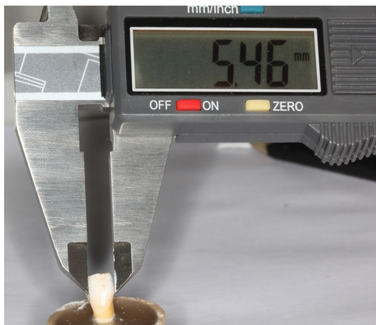
Figure 3 Definition of the amount of stripping.
