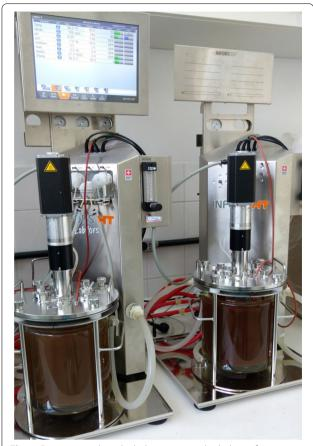
**Fig. 2** Reactor vessel in which the enzymatic hydrolysis of steam-treated substrates were carried out at 20 wt%TS using Cellic CTec3
