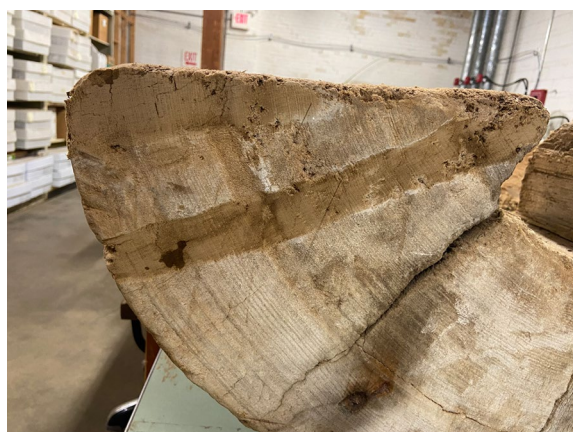
Fig. 3 Overlapping radii sanded to distinguish annual rings for radiocarbon wiggle-match and dendrochronological dating
