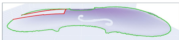
Fig. 9 Contour of the sound board (green) with highlight on the raised part to be manually removed (red)
