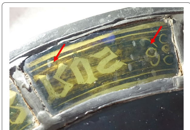
Fig. 5 Elongated bubbles arranged in straight and parallel lines suggesting the Ca-rich yellow glass pieces were produced with the cylinder forming technique. As an example, we picture the exterior side of the piece 25 from panel AV.1165, in reflective light
