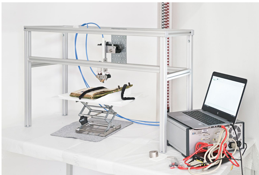
Fig. 2 FORS analyses of the Vienna Moamin. A lifting platform was used for the adjustment of the measuring position and the adequate distance. The fiber optic probe was mounted on a tetrapod, which also served to mount the rFTIR instrument
