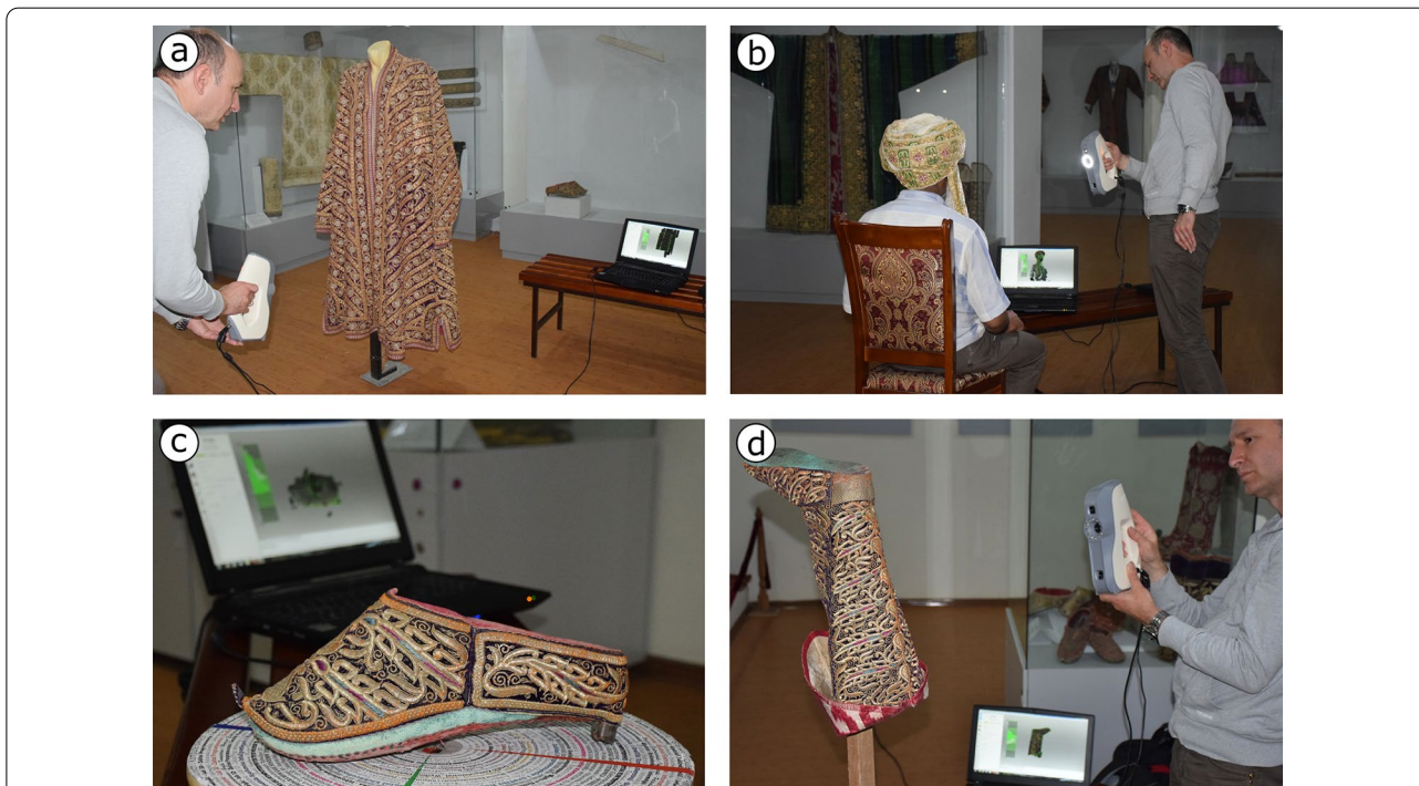
Fig. 6. 3D SLS of the elements of the Emir’s costume: a dressing gown, b turban—salla, c kaushi—low shoe and d mahsi—high shoe
