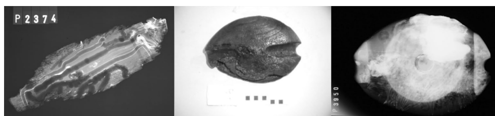
Fig. 3 X-ray images of waterlogged wooden artefacts from wreck sites. Left: a barrel stave fragment from the “Stirling Castle”, wrecked in 1703. Regions of low density caused by marine wood borer infestation can be clearly seen. Centre and right: a photograph compared to an X-ray scan of an elm pulley block from the “London”, wrecked in 1665. X-ray analysis reveals internal features and regions of high/low density not otherwise visible. (Images courtesy of Angela Middleton, copyright Historic England)
