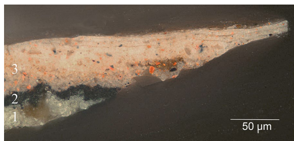
Fig. 14 Detail of cross-section sample 1 from flesh highlight, proper right hand, showing: (1) imprimatura (2) black background paint layer (3) flesh highlight paint layers. Several extraordinarily thin layers of cooler and paler pink paint, each approximately 4–5 micrometers thick, are seen uppermost
